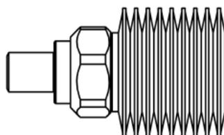
Smear loctite 572 over nose of bellows, thread nut onto bellows ensuring the thread starts squarely. Grip bellows lightly by hand and tighten the nut with a 1" A/F spanner until the nut contacts the bellows shoulder.
