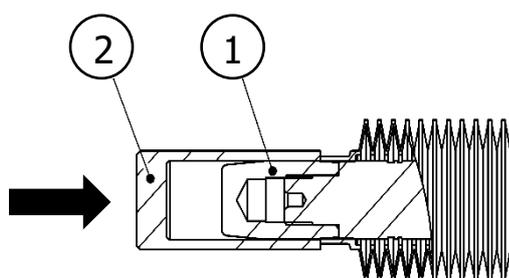
Screw Item No. 2 (assembly spigot) onto the piston shaft
