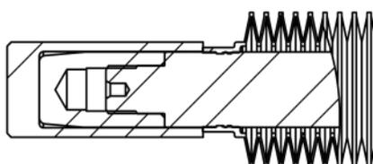
Using Item No. 1, push bellows over spigot until located in groove.
